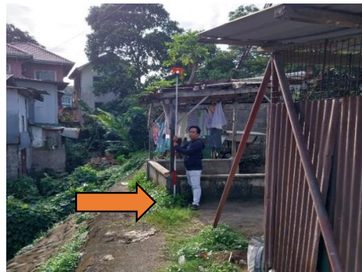
Above right pic (7) Shows the location of the TBM where the x-sect measurement was referred to, at the LB, u/s side of the hanging bridge.
