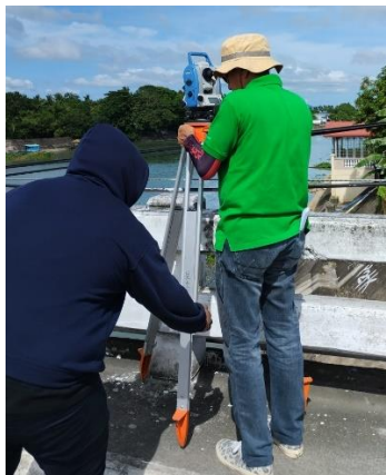
Below right pic (18) River surface velocity measurements being carried-out atop the Lumban Bridge (station 3).
