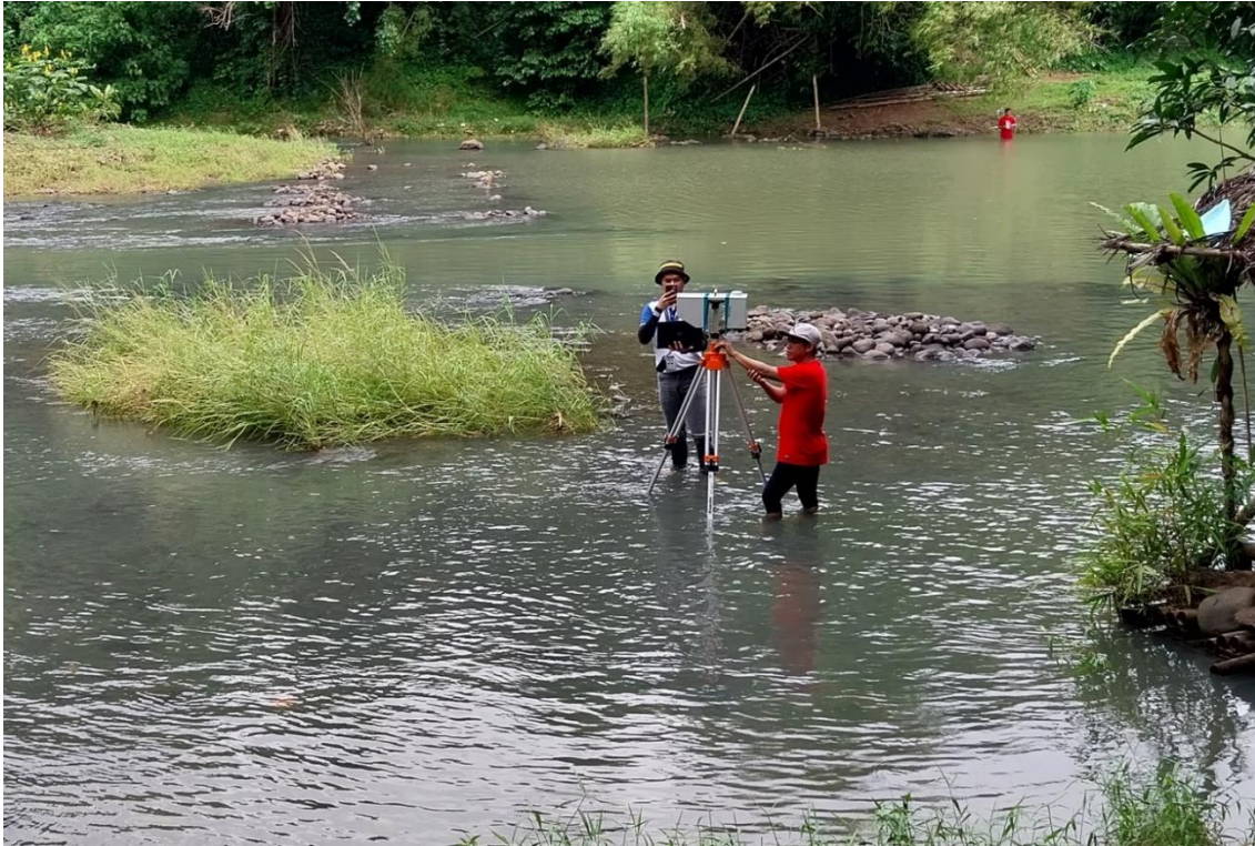
Above pic (14) Taking river surface velocity measurements by wading along the shallow portions of Pagsanjan River in station 1.
