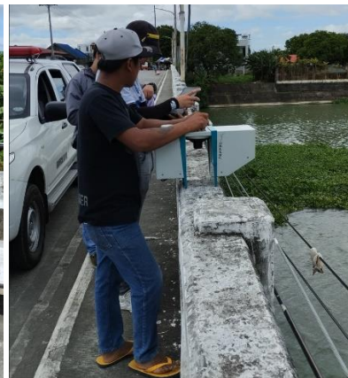
Below right pic (18) River surface velocity measurements being carried-out atop the Lumban Bridge (station 3).
