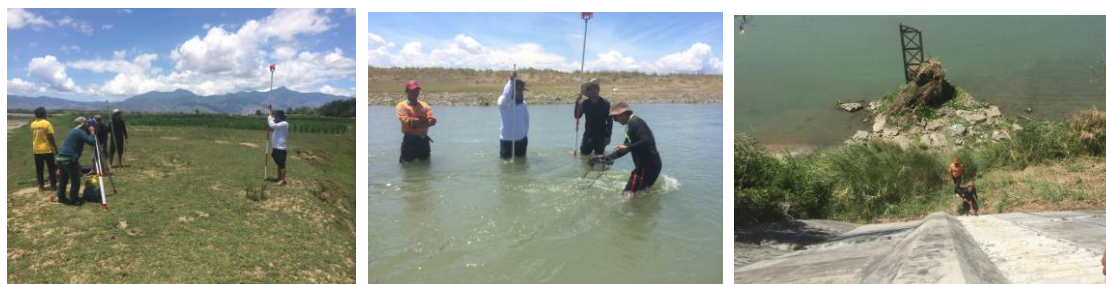
Top pictures: River cross-sectioning and river velocity measurements by wading at Sapang Buho, upper Pampanga River forecasting point, together with personnel of Palayan City DRRMO;
