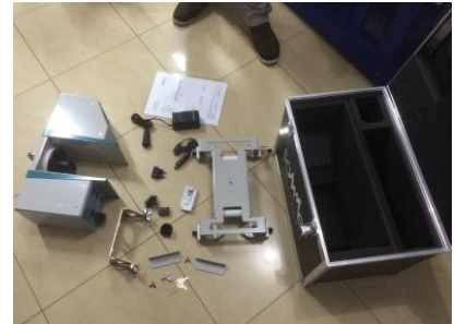
A newly acquired radar profiler (RP-30) to facilitate river velocity measurements of the center.
