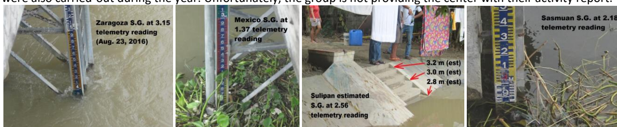
Top left: Zaragoza staff gauge (S.G.) at a reading of about 3.90 meters and a telemetry reading of 3.15 meters at time of WL validation trip; for now the station's WL telemetry reading has yet to be readjusted by HMTS. (Above, 2 nd , 3 rd & 4 th pictures) The Mexico, Sulipan and Sasmuan staff gauges at the time of WL validation surveys. All 3 stations were readjusted last September.
