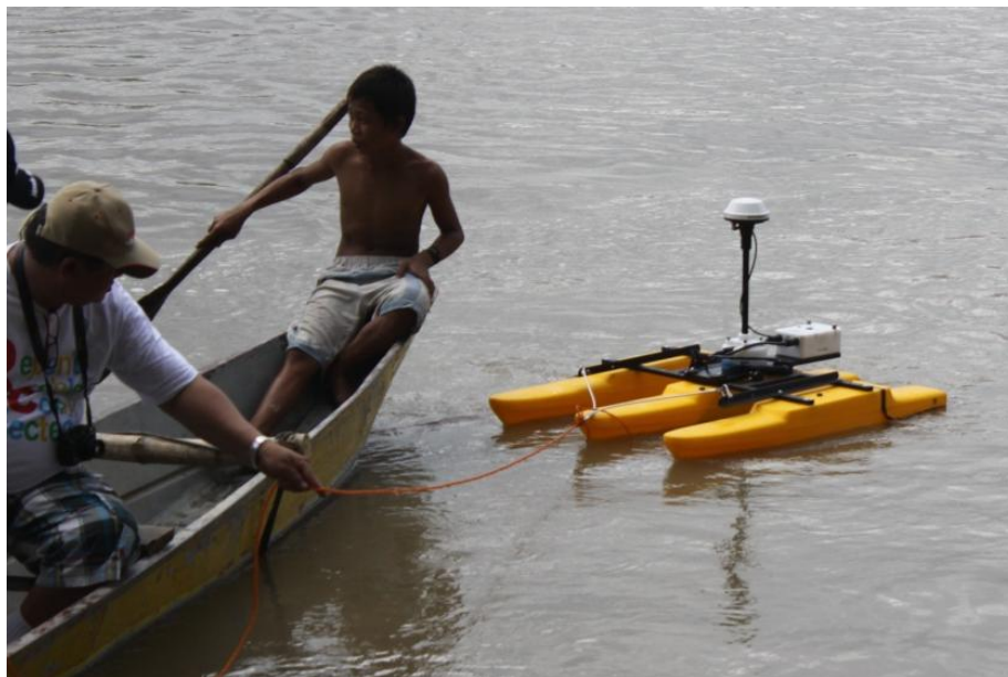
Figure 3. Tethered ADCP boat used for making discharge measurements attached to a manned boat
