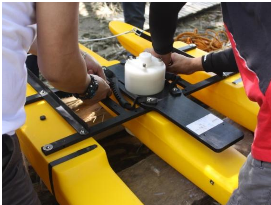
Figure 2. Assembling the ADCP instrument.
