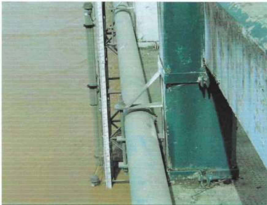
Pic 9.0 San Isidro streamgaging station at 2.90 meters reading at around 1300H, 23 Nov. 2004, several hours after reaching its peak of more than 3.15 meters. The first sensing was totally submerged during the peak stage.
