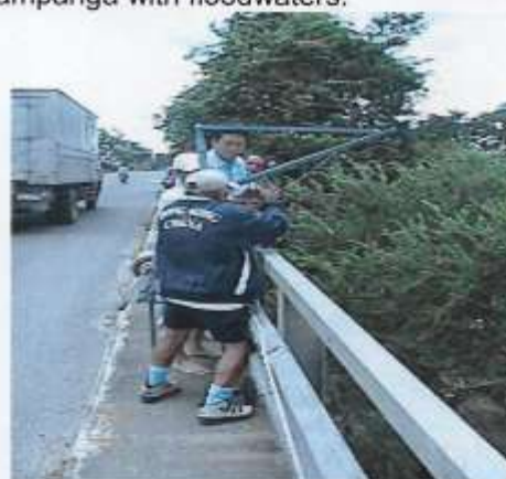
Pic 29.0 River velocity measurements undertaken at Arayat gaging station 2 days after the flood event (Aug. 31, 2004).
