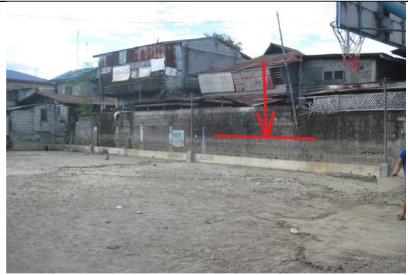
Sulipan station: Basketball court beside the station with flood level height at a station's S.G. reading of 4.5 m (estimated)
