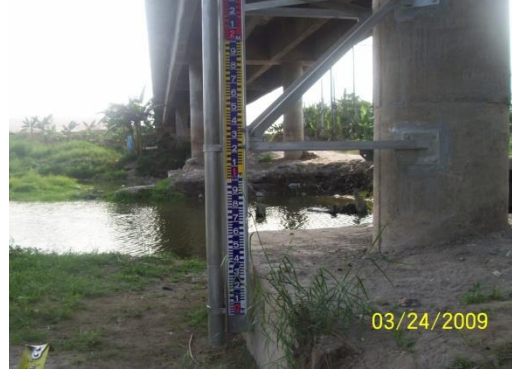
The S.G. and station sensor is located at the middle bridge pier
