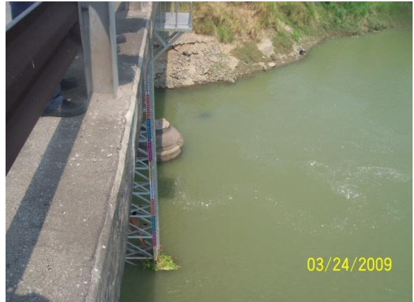
Top: A frontal view of the Arayat RR-WL telemetry station housing; picture below shows the S.G. and sensor platform for the said station.
