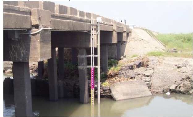
Top: A view of the station at a relatively dry period. Below is the sensor and S.G. platform at the bridge beside the station (old location).
