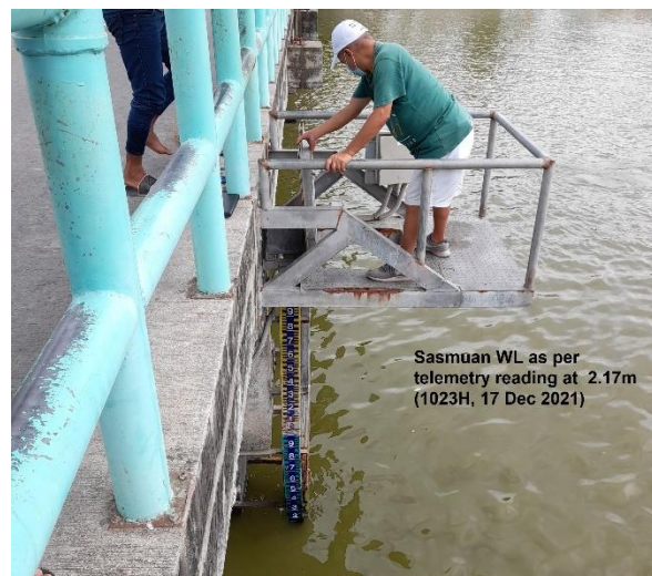
Pic 14 Checking and validating the River WL at Sasmuan stream gaging station on 17 Dec 2021.
