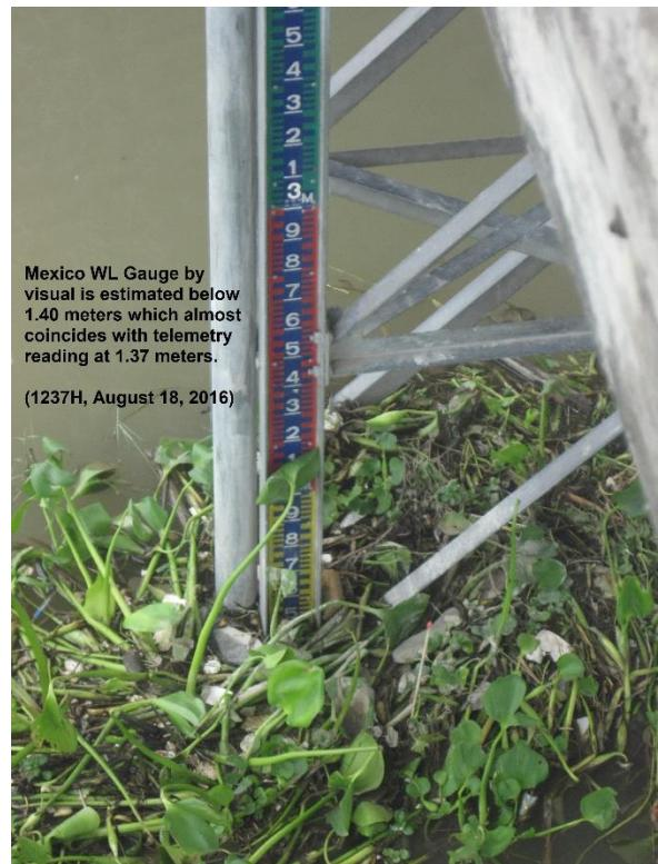
Mexico WL Gauge by visual is estimated below 1.40 meters which almost coincides with telemetry reading at 1.37 meters.
