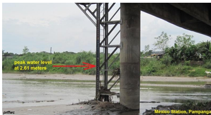
(Top) The Abacan River at Mexico station crested at 2.61 meters during Habagat 2013. (Right) A resident of Bgy. San Agustin, Candaba points to the peak floodwaters reached in the area's flood marker in their barangay during Habagat 2013.
