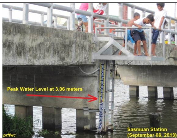
River stage recorded at Sasmuan water level telemetry station crested at 3.06 meter on August 21, 2013.
