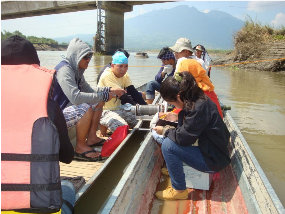
Figure 5. Current meter method by boat
