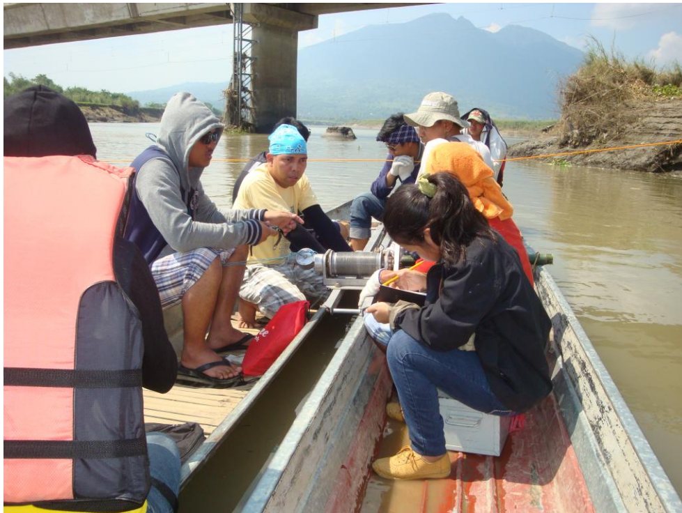
Figure 7. Current meter method by boat.
