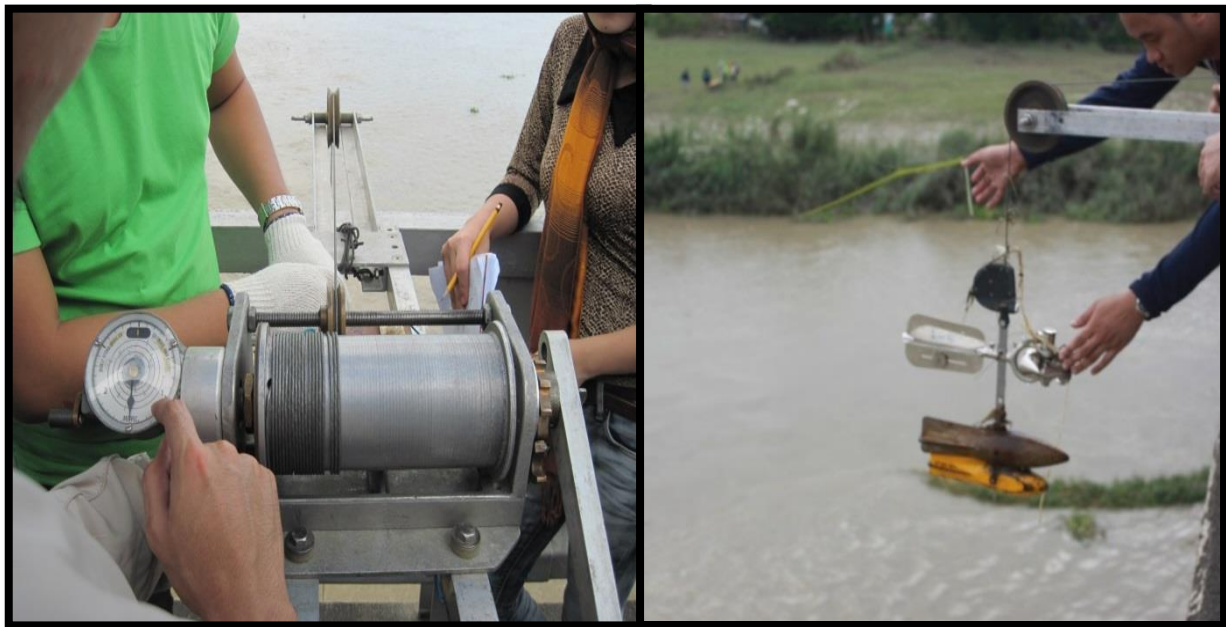
Figure 2. Actual Setup of the Price AA Current Meter
