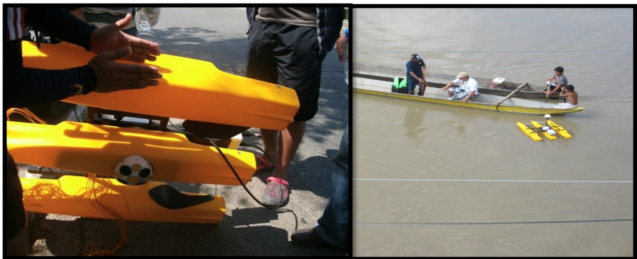
Figure 5. Actual Setup of the Acoustic Doppler Current Profiler (ADCP)
