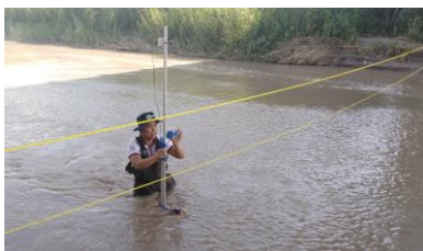
(L to R) PRFFWC personnel with Hyquest training staff during the specialized Stream Gaging workshop for DPWH using "Redback" current meter; river velocity measurements during the training's fieldwork (Jul 08-09)
